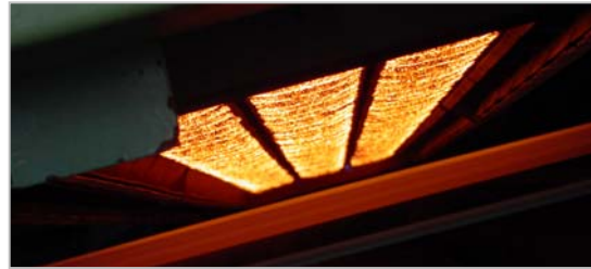
Metal fiber emitter for the paper coating drying (By ACOD, Inc.)
