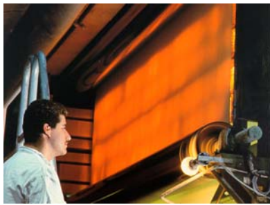
Metal fiber emitter for the paper coating drying process (6.5 kW)
