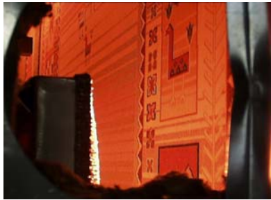
IR pre-dryers in coloring lines prior to hot flues (100 ~ 250 kW/m 2 )
